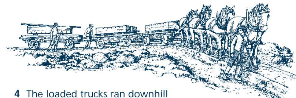
4 The loaded trucks ran downhill from Haytor to Ventiford on the Stover Canal, but they had to be brought uphill from Holwell Quarry. Teams of horses were used to pull trains the short distance up from Holwell to the point where gravity could take over. The trucks had no brakes but braking was carried out by levering long poles against the wheels.
