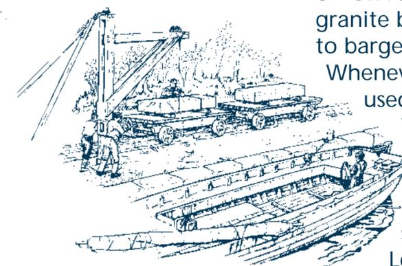
6 On reaching the canal, the granite blocks were transferred to barges using a wooden derrick. Whenever possible, sails were used to power the barges. The barges transported the granite to Teignmouth where it was transferred to cargo ships for the journey to London and elsewhere.
