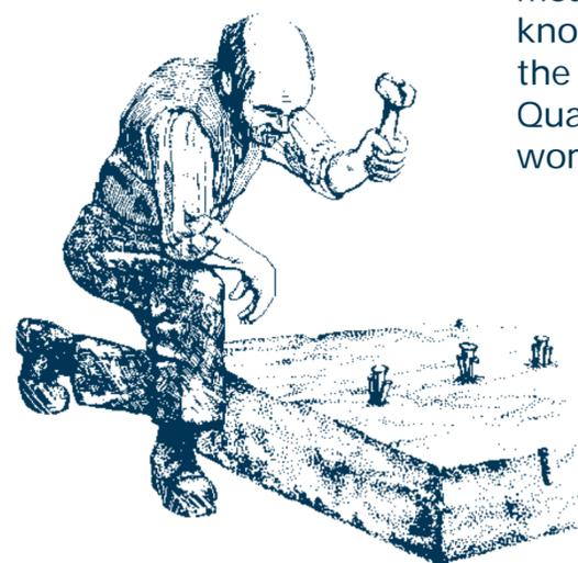
2 Once the line of holes was drilled, a tapered plug called a *tare* was driven into each hole between two curved slivers of metal known as feathers. By tapping on each of the tares in turn a line of stress was formed causing the block to split along that line.
